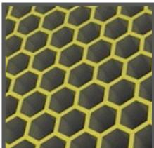
The high-tech ceramic energy accumulator with a regeneration efficiency of up to 97% ensures heat recovery from the exhaust air to heat or cool the supply air flow. Due to its cellular structure, the unique regenerator has a large air contact surface and high heat conducting and accumulating properties.
