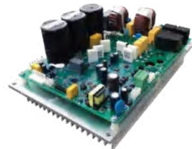
Intelligent IPM DC frequency conversion chip realizes the automatic adjustment and intelligent control of high and low frequency operation of compressor, and comprehensively improves the stability and high energy efficiency of the system.
