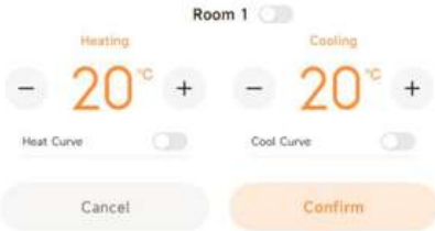
Room temperature control (Heating/Cooling Target room temperature in Zone 1)
